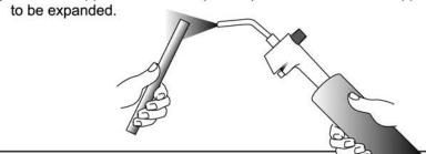
2) Debur the inner walls of the tubing completely and make sure the tube will fit easily over the expander head. DO NOT FORCE THE TUBE OVER THE EXPANDER HEAD!
