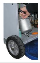
Clean with compressed air or replace the cartridge if necessary.
