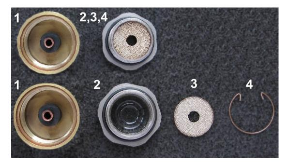
After dismantling of the upper part (No. 2, 3, 4) withdraw the blocking spring (No.4) and dismantle all single parts (No. 2, 3, 4), which has to be cleaned including the sight glass interior (No. 1).
