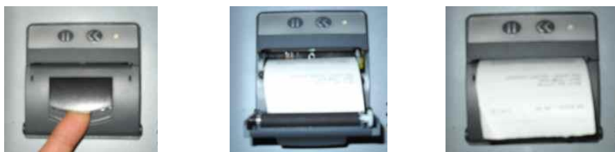
Fig. 8 - Procedures for paper replacement
