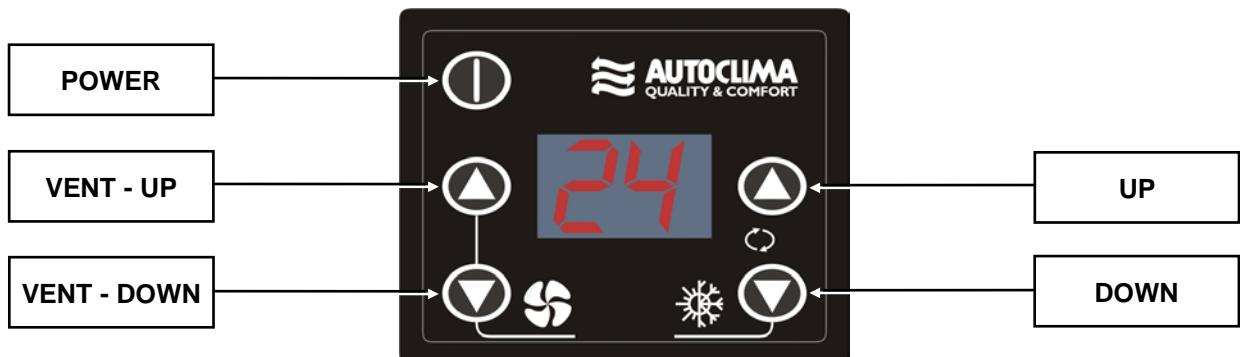
The Control Panel in the driver's panel has the main CPU and it is composed by a keyboard for the conditioning air system's operational programming, and also by a numerical display for the visualization of parameters, operational status and temperature.
